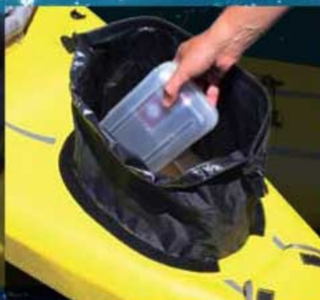
New Rear Storage Access Hatch
